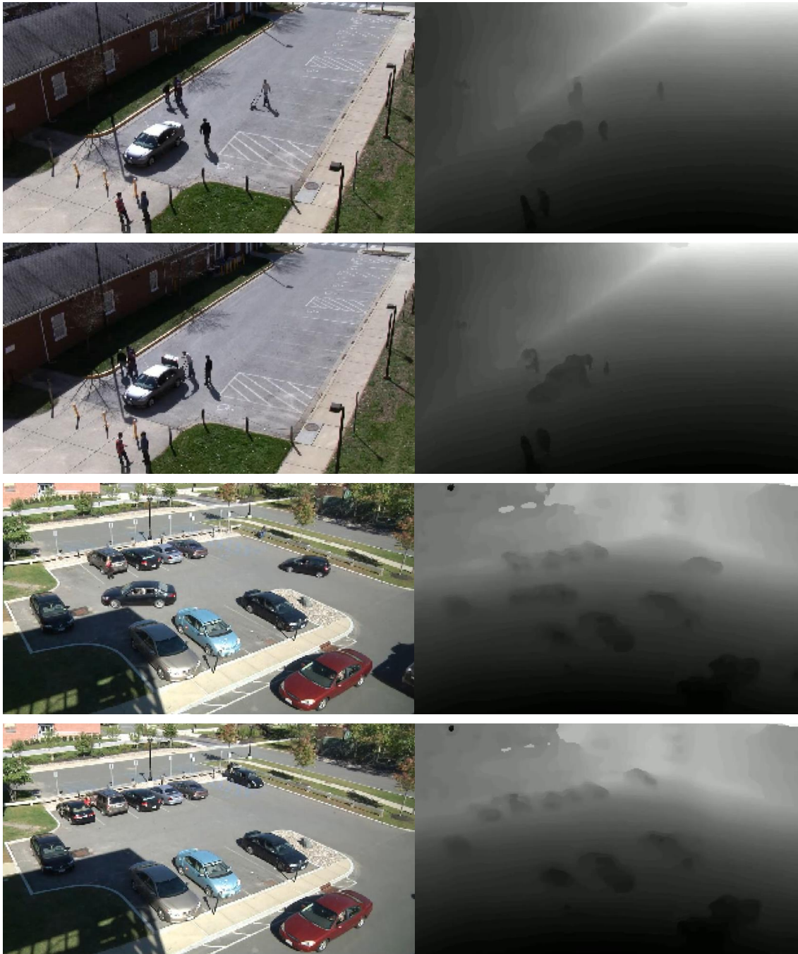
Figure 6.4: Depth estimation output from an FCN trained on data generated by ADR for VIRAT
